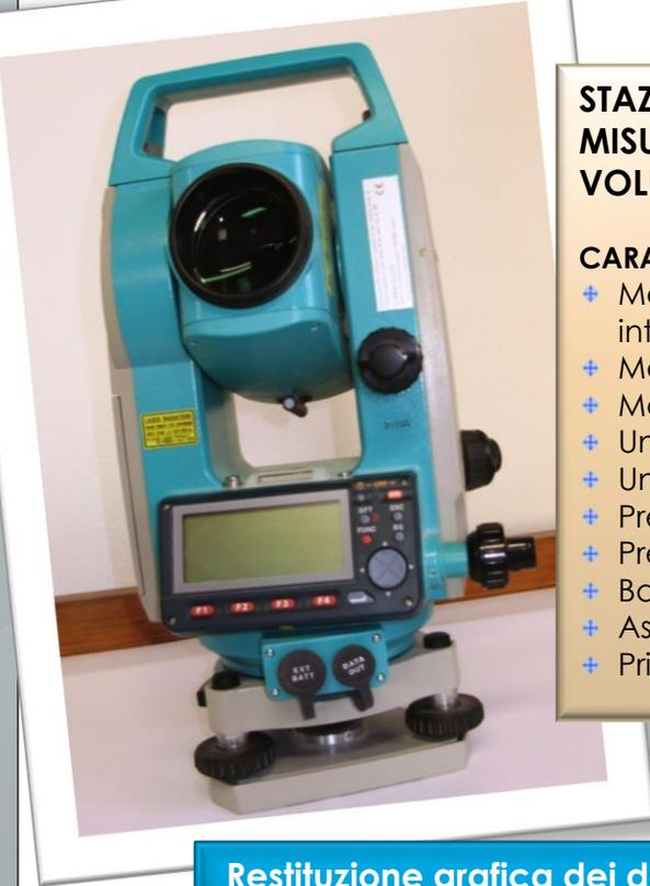
**STAZIONE TOTALE PER RILIEVI TOPOGRAFICI, MISURE DI PRECISIONE, CALCOLO DI AREE E VOLUMI**
